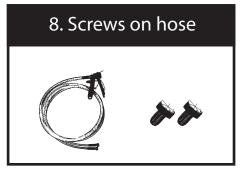
If hoses are not being used for some time, shut off by using the 2 screws. That way, air and oxygen cannot enter the hoses.
