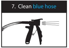
Flush blue hose by turning ball valve from the CKA open and pulling the trigger.
