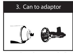
Connect the PU cleaner can to the Clean Kit Adaptor (CKA). Make sure CKA valve is closed (vertical, as on drawing above).
